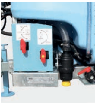
Scarico ecologico / Ecological drain / Kit rinçage ecoplus (retour sur aspiration) / Ökologischer Ablauf / Escape ecológico
